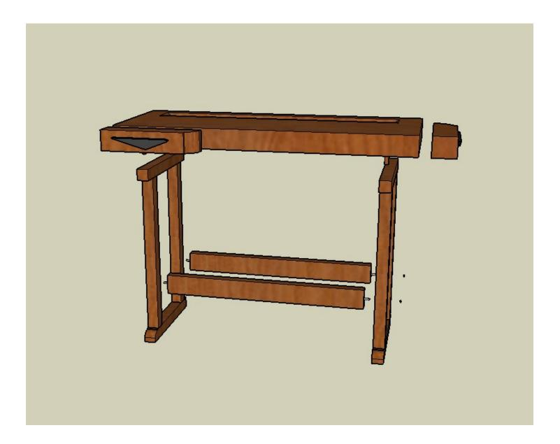
The workbench base "bolts" together with just 4 nuts and washers.
